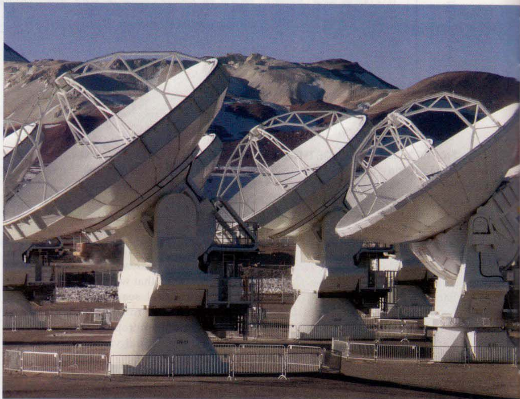
FIGURE 1. ANTENNAS FROM THE ATACAMA LARGE MILLIMETER/SUBMILLIMETER ARRAY are on an elevated desert plateau ideal for measuring wavelengths from the far-IR to radio. The 66 antennas can cluster together for higher-sensitivity measurements or spread over tens of kilometers to zoom in on details. (Courtesy of W. Garnier/ALMA/ESO/NAOJ/NRAO.)
